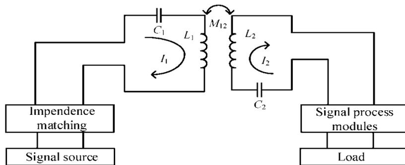
Fig (1): the equivalent box diagram of the wireless charging system
