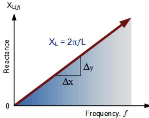
Fig(3): Inductive Reactance against Frequency.
