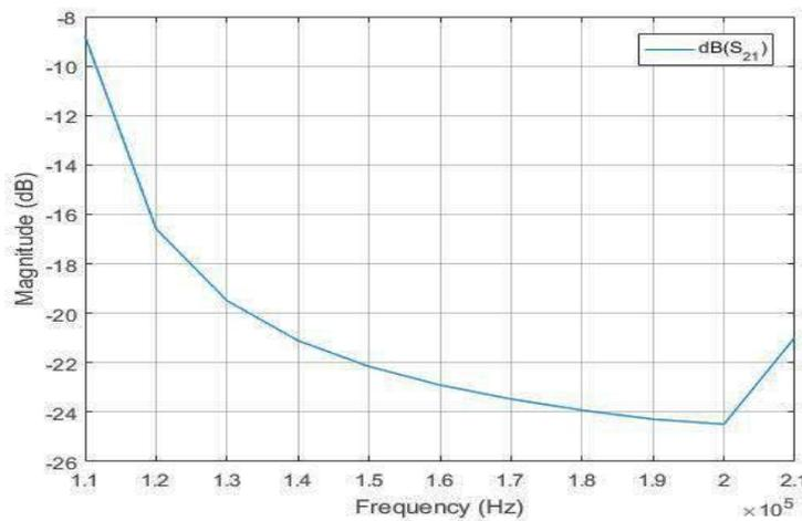
Fig(12):  $S_{21}$  parameter Vs. Operating frequency at 20 mm spacing.
