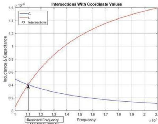
Fig(11): Calculated Resonant Frequency Point
