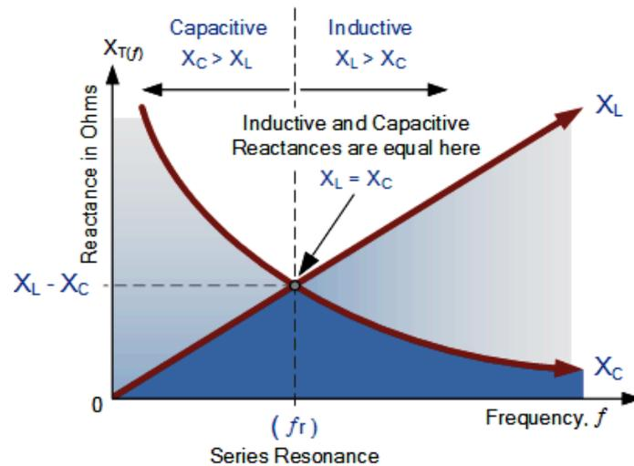
Fig(5): Series Resonance Frequency at  $f_r$ .
