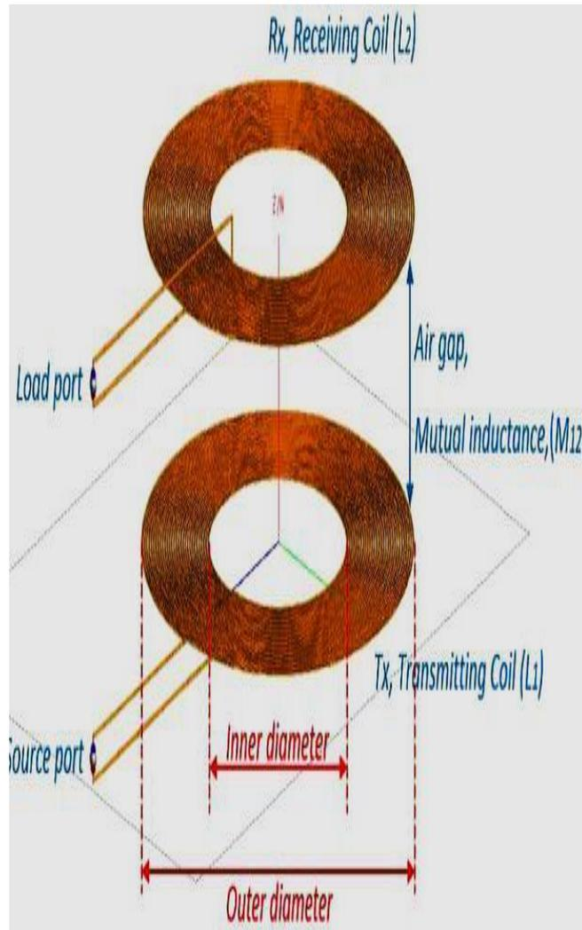
Fig (6): Resonant Coupling Coils.
