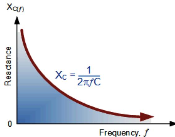
Fig(4): Capacitive Reactance against Frequency.
